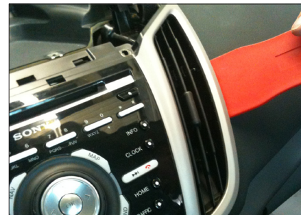
13. Unclip air vents Remove air vents
